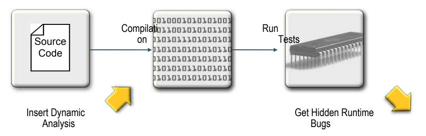
The tools insert some analysis code at every line of source code; They build a database of all program elements, and then at runtime, the tools check each data value and memory reference against its database to verify consistency and correctness
