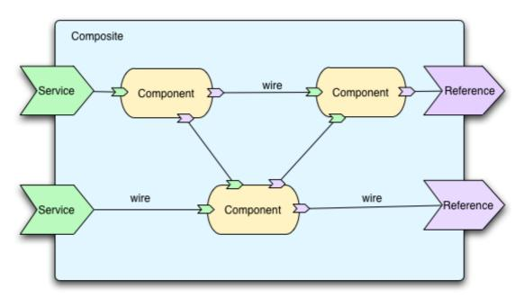
On this diagram the internal links represent wires between services and references within a single component.
