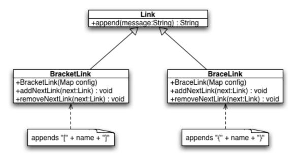
At the start of the demo, the Java classes which define the composites and the Link interface they implement are unknown to the Newton container. All are loaded dynamically as the composites are installed.
