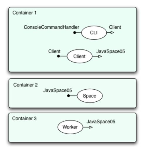
As the composites are created Newton examines the their services and references and uses them to dynamically wire up the composites in the following arrangement.
