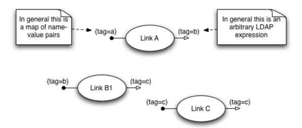
As the composites are installed Newton examines their external interfaces, attributes and filters, and uses these to organize them into a chain as below
