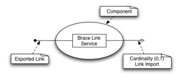
Here the component is based on an instance of the ExportingBraceLink class. It provides a service called link, which is obtained by calling the instance's \_exportLink() method The multiplicity of (0,1) on the reference means that the composite wants to connect to at most 1 Link interface, but can still function if it can't find any. The wires link the service and reference to the concrete component.
