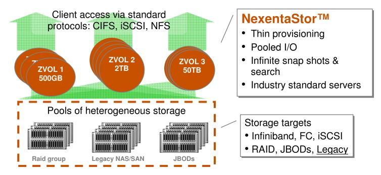
NexentaStor abstracts the underlying storage, creating ZVOLs that are exposed to clients via standard protocols. These ZVOLs can be managed via infinite snap shots and block level replication with the assistance of integrated search. No special client software is required. The result is a breakthrough is ease of use, price / performance, and price / capacity.
