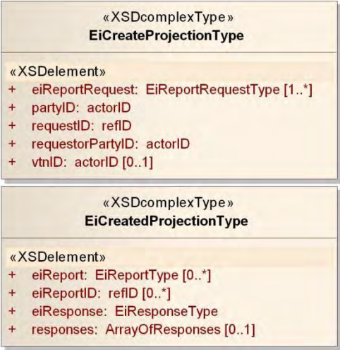
1784 1785 Figure 10-6: UML Diagram of Projection Payloads
