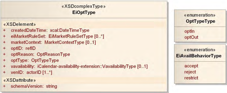
1876 1877 Figure 11-5: UML Class Diagram for EiOpt Type
