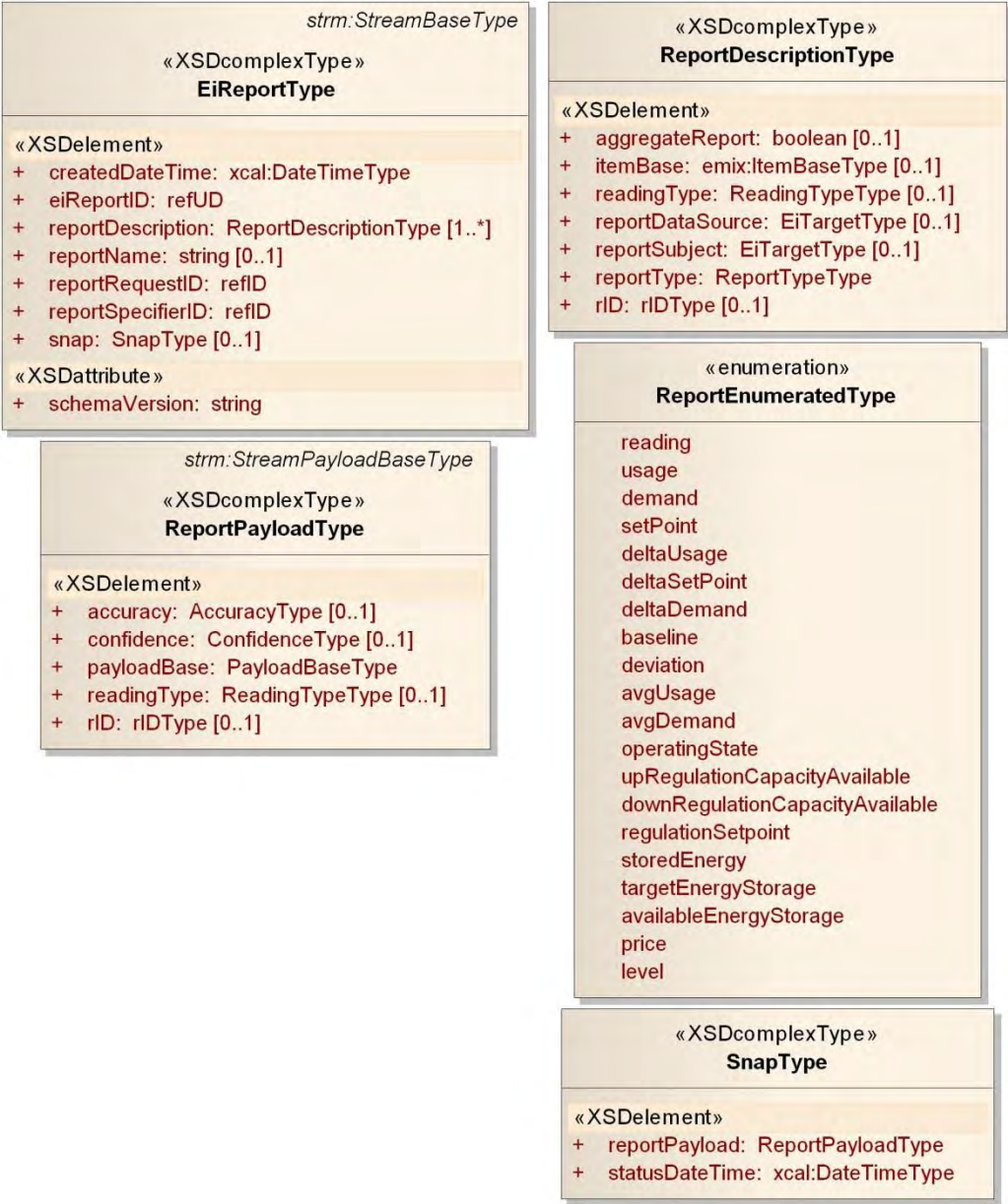
1246 1247 Figure 5-16: UML Class Diagram of Reports
