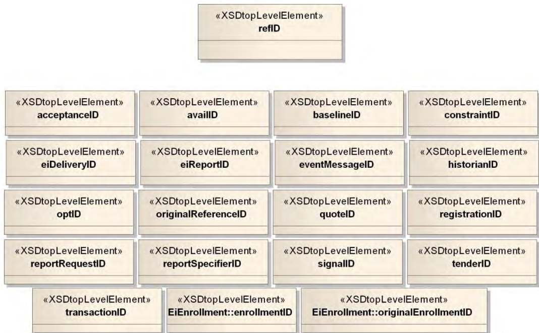
Figure 5-17: UML Diagram showing refID and its derived types
