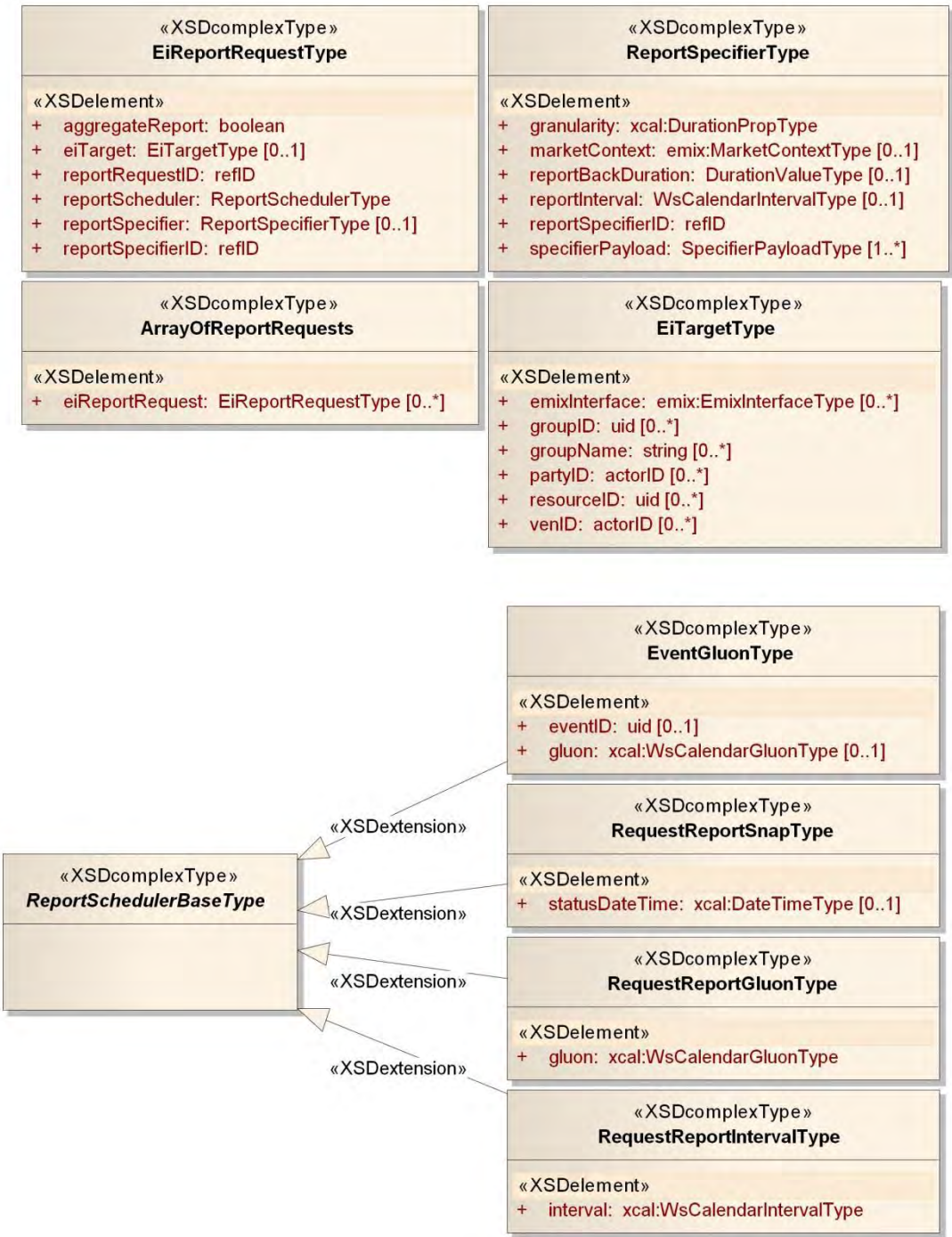
1185 1186 Figure 5-11: UML Class Diagram of Report Request
