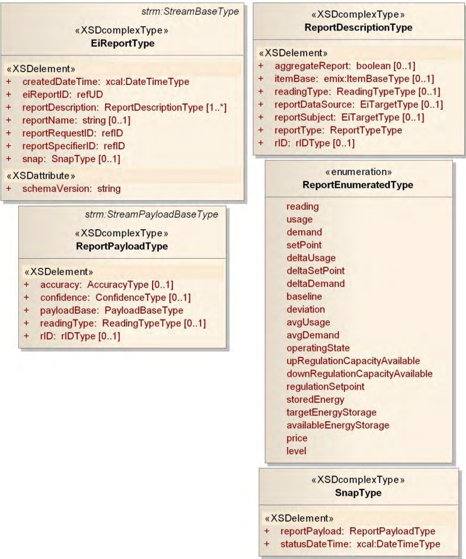
1789 1790 Figure 10-7: UML Class Diagram for the EiReport Class 1791
