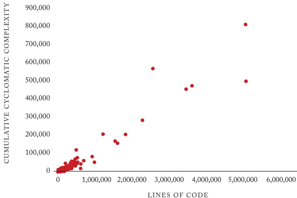
Coverity Prevent captures the Cyclomatic complexity and Halstead effort calculations for each function that it analyzes. Since the algorithms for both of these metrics include factors that increase with the amount of code, it is not surprising that the total complexities for both metrics are significantly related to the size of the code base that they are calculated for.
