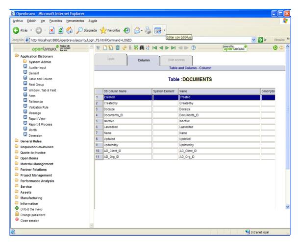
These columns are assigned a reference (which defines the data type) depending on its name and data type. A System Element is automatically assigned, the name of this element is the same as the column, if exists an element matching this rule is associated otherwise a new one is created.
