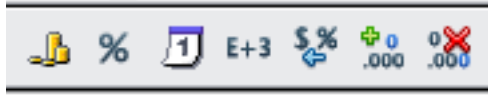
Figure 38: Number format icons. Left to right: currency, percentage, date, exponential, standard, add decimal place, delete decimal place.
