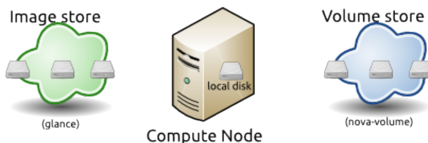
Figure 2.1. Base image state with no running instances
