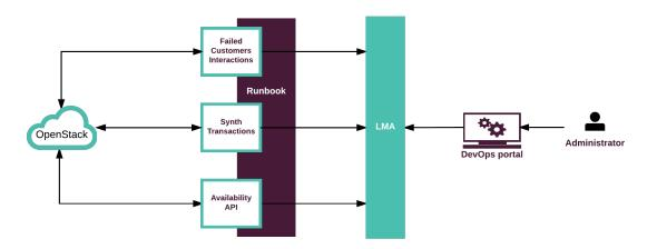
Runbook executes FCI, synth transactions and API tests and stores the corresponding data in the Logging, Metering, and Alerting (LMA) toolchain. The DevOps portal queries LMA and creates graphs and heatmaps for the cloud status. The cloud operator monitors the heatmaps and graphs through the DevOps portal.
