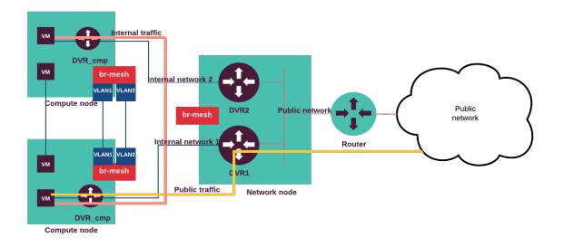
The internal traffic from one tenant virtual machine located on the virtual Internal network 1 goes to another virtual machine located in the Internal network 2 through the DVRs on the
