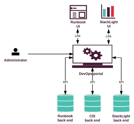
The following diagram shows a high level architecture of the DevOps portal components.
