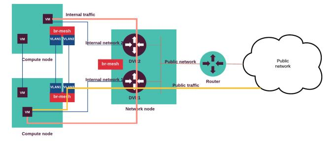
The following diagram displays internal and external traffic flow.
