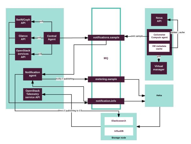
Tenant Telemetry uses the Ceilometer agents to collect data and Heka to transfer data to InfluxDB and Elasticsearch. The Ceilometer API is used to retrieve data from back ends and provide it to the end user.
