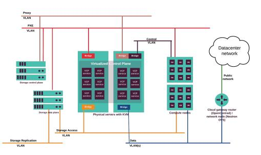
In an OpenStack environment, you typically work with the following types of networks:
