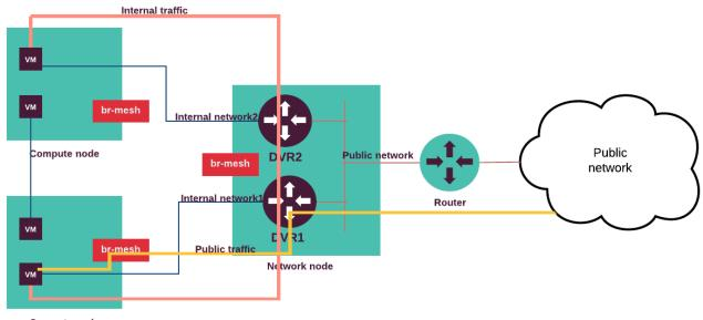
The following diagram displays internal and external traffic flow.
