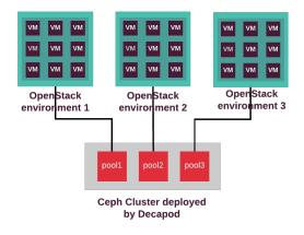
Decapod uses Ansible with the Ceph-Ansible community project to deliver the best user experience. For tasks, you can use plugins that encapsulate the appropriate settings. You can customize any configuration before execution.
