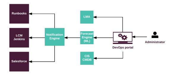
The Forecast Engine sends notifications with the required actions, such as add more nodes or clean up the storage, and creates a ticket in the corresponding task management system, such as Salesforce. The Forecast Engine pulls data from LMA and CIS and predicts the future resource utilization. The cloud operator accesses graphs and heatmaps through the DevOps portal that displays the capacity of the cloud.
