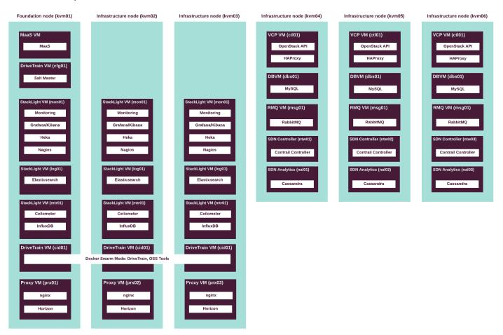
The following diagram displays the infrastructure and foundation node services mapping for tenant networking with Neutron Open vSwitch.
