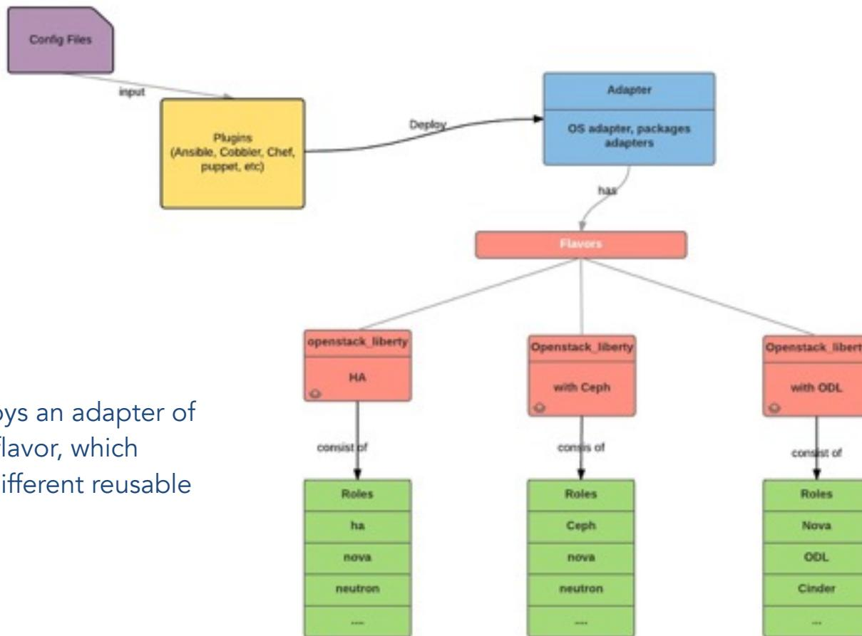
Plugin deploys an adapter of a particular flavor, which consists of different reusable roles
