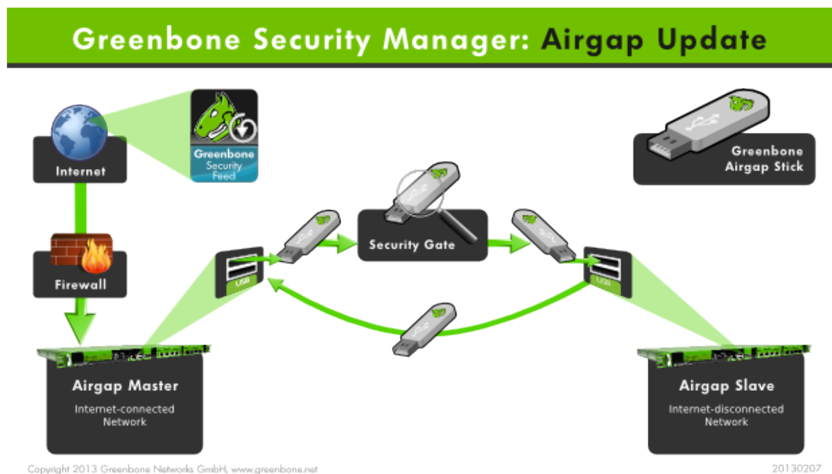
Fig. 6.18: The Airgap function allows for the update of GSM that are not connected to the Internet.
