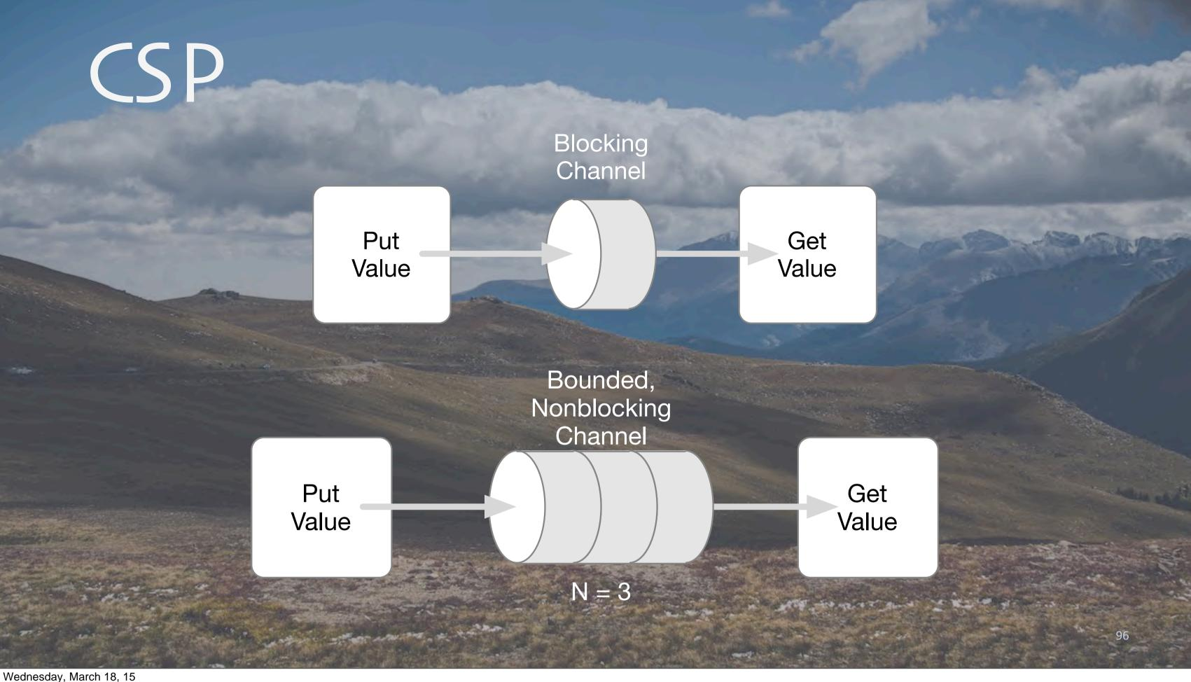
Schematic view of simple CSP interactions. If the channel queue has one slot, then it's blocking; the "putter" wait for a "" "" "getter" to be on the other side. If there are >1 slots, the putter won't block unless all the slots are full. See my talk on error handling in reactive systems where I discuss CSP in more detail. (I'll discuss CSP vs. Actors in more depth in my other talk.)
