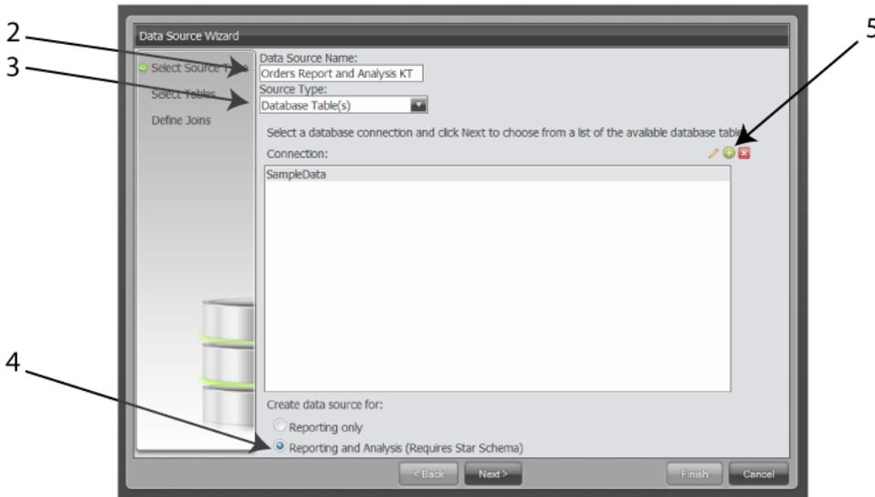
6. In the **Connection Name** text box, type **SampleData**. A Connection Name must be easy to remember and must identify the data you are accessing. The name can have spaces but it cannot have special characters (#, \$, %, etc.).
