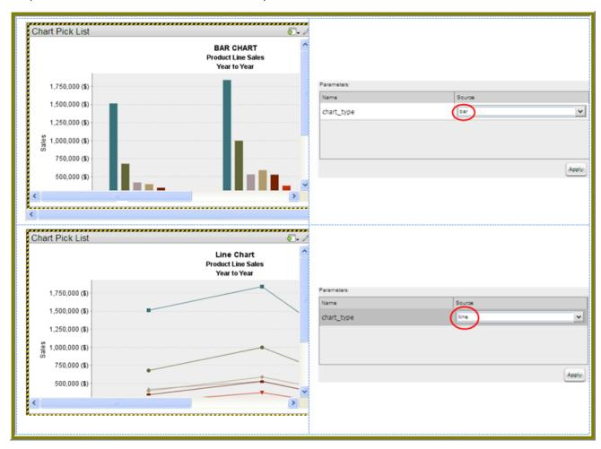
Parameter names are "hard-coded," in the file; that means they cannot be changed. Neither can you change the number of parameters associated with a file. When you create a chart using the Chart Designer, embed a URL into a dashboard, or create a data table, you can change both the name and value of a parameter.
