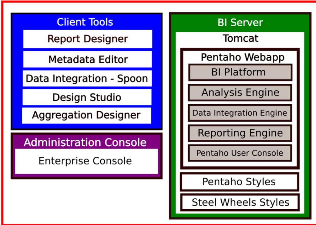
**The BI Suite** is all of the software inside of the red box. It's the BI Server plus standalone client tools and a graphical interface for managing data sources, users and roles, and other administrator functions (the Pentaho Enterprise Console). Enterprise Console is an extension of the open source Pentaho Administration Console; it is only available to Pentaho Enterprise Edition customers.
