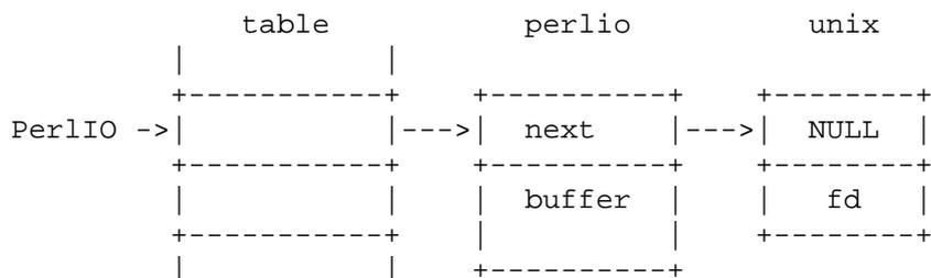
The above attempts to show how the layer scheme works in a simple case. The application's `PerlIO` \* points to an entry in the table(s) representing open (allocated) handles. For example the first three slots in the table correspond to `stdin`, `stdout` and `stderr`. The table in turn points to the current "top" layer for the handle - in this case an instance of the generic buffering layer "perlio". That layer in turn points to the next layer down - in this case the low-level "unix" layer.
