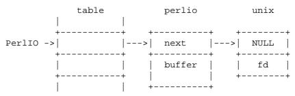
The above attempts to show how the layer scheme works in a simple case. The application's Perlio \* points to an entry in the table(s) representing open (allocated) handles. For example the first three slots in the table correspond to stdin,stdout and stderr. The table in turn points to the current "top" layer for the handle - in this case an instance of the generic buffering layer "perlio". That layer in turn points to the next layer down - in this case the low-level "unix" layer.
