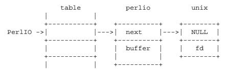
The above attempts to show how the layer scheme works in a simple case. The application's Perlio \* points to an entry in the table(s) representing open (allocated) handles. For example the first three slots in the table correspond to stdin,stdout and stderr. The table in turn points to the current "top" layer for the handle - in this case an instance of the generic buffering layer "perlio". That layer in turn points to the next layer down - in this case the low-level "unix" layer.
