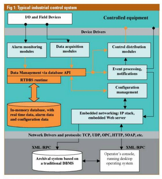
This diagram represents the data-centric view of the control process: data collected by sensors in the form of input signals is stored in the real-time database. Output signals are generated by the controller's data management services and are delivered in real-time through the control distribution modules to the controlled equipment (assembly line, motor, generator, combustion engine, etc), to support critical processes.
