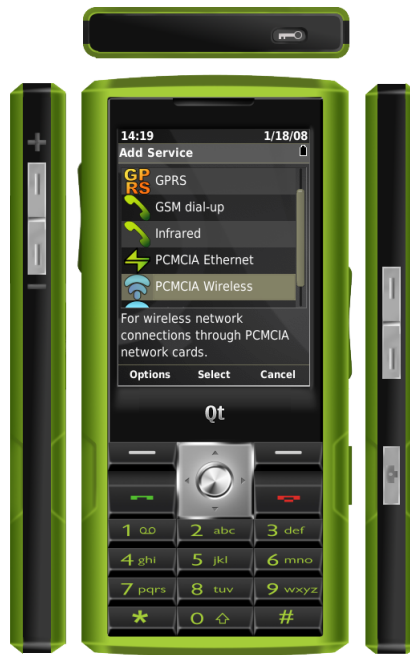
Figure 9: An example QVfb session using the Greenphone skin supplied with Qt Extended, showing the buttons on each side of the device.
