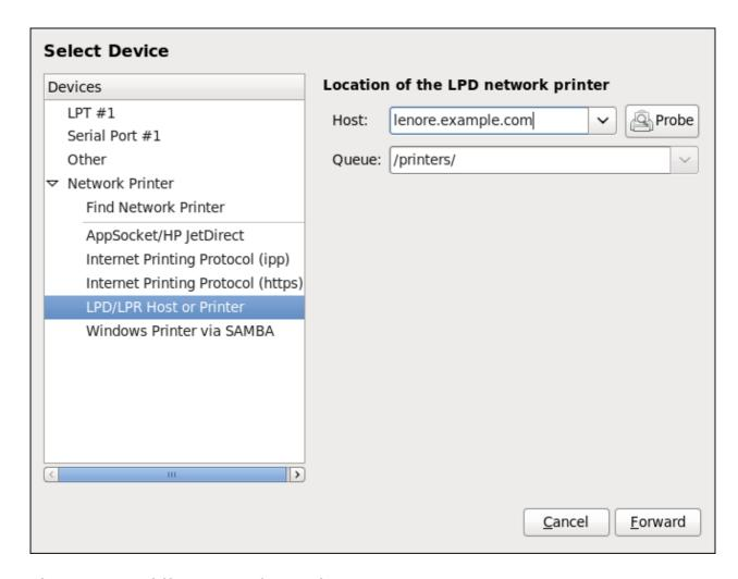
Figure 14.7. Adding an LPD/LPR printer
