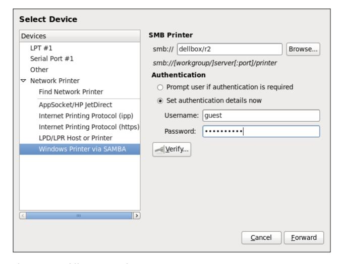
Figure 14.8. Adding a SMB printer
