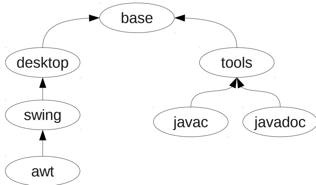
*Example to illustrate how Jigsaw can potentially break down components*
