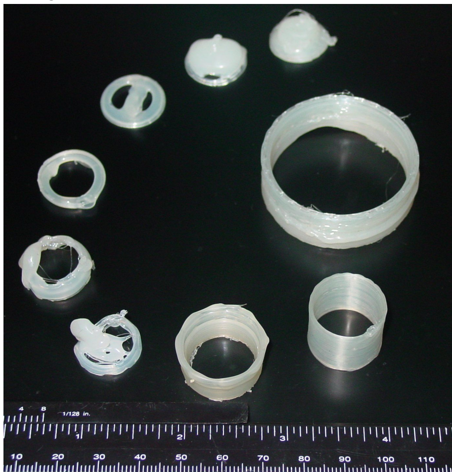
Figure 10 Various deposited EVA cylinders, arranged approximately chronologically.
