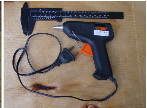
Figure 7 The NZ$2 glue gun used for these experiments. It takes 7mm glue sticks, consumes 10W 110/240VAC. Max. tip temp. \approx 110^{\circ}\text{C} , 1mm nozzle exit.
