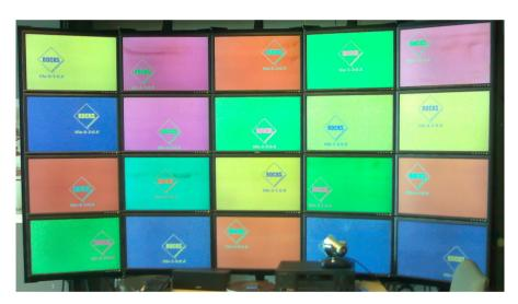
After all the tile nodes have been installed, you'll need to configure a file that describes your videowall. If your wall is built for one Tile node for each LCD Display follow the instruction in the next section. Otherwise skip to the subsequent section to configure your wall in TwinView mode.
