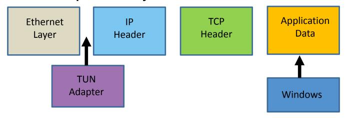
Using a TUN Adapter allows the IP and TCP headers to be replaced
