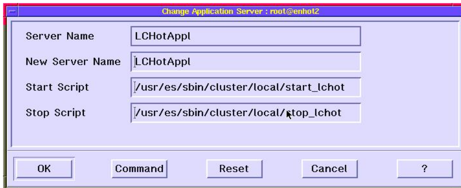
Figure 28: HACMP Application Server - Example for Hot-Standby
