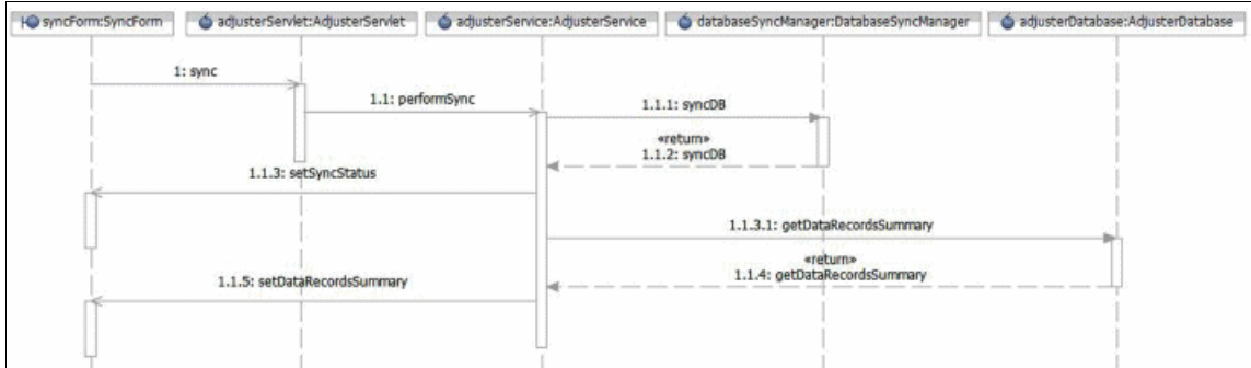
Figure 9-6 UCR_3-9RetrieveSendClaimData sequence diagram
