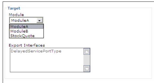
Figure 9-12 Changing an SCA binding using the administrative console
