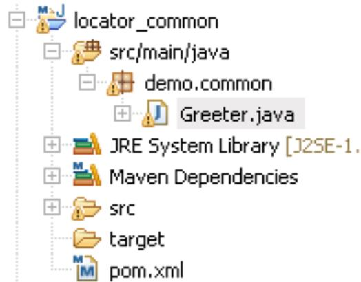
4. The common application will be deployed as an OSGi bundle. So we'll need to edit the pom.xml. (Please refer to [Section 2.2.3, "Making SOAP calls with soapUI"](#) for details.)
