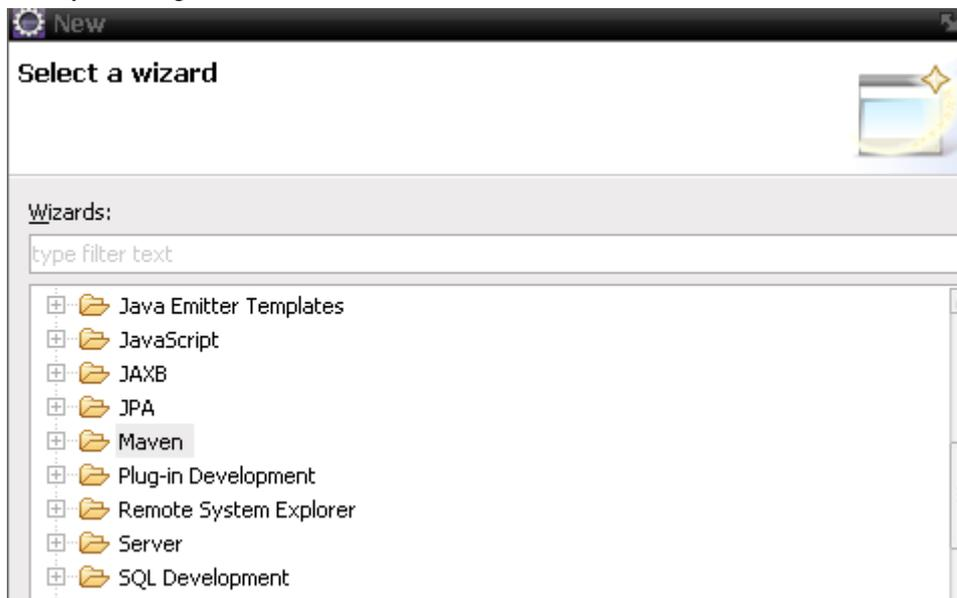
By default Eclipse's embedded Maven is used. However, it's recommended to use the external Maven you downloaded and installed in the previous step. Open Main Menu "Window -> Preferences -> Maven -> Installations" to change the default setting:
