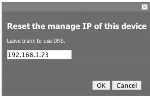
3. Enter the new IP address for the device. Alternatively, leave the field blank to allow the IP address to be set by DNS.
