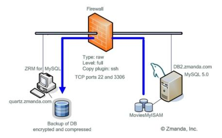
Fig. 3 Raw backup with SSH connection.
